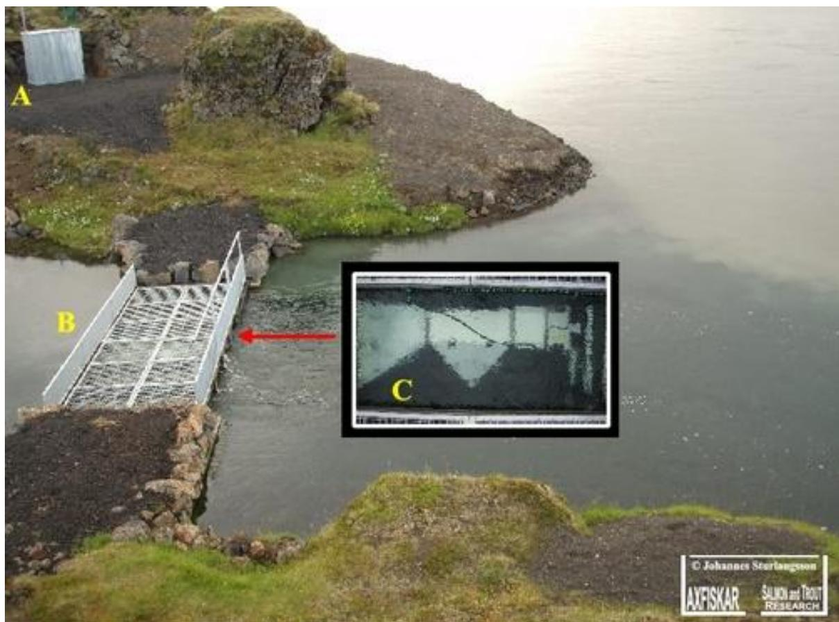
**Fig 3.** The counter facility unit in the mouth of River Tungulaekur where it opens into the glacier river Skafta. The little building (A) is for storing computers and other equipment for
